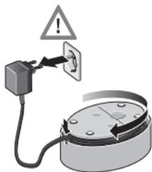
If you do not need the full length of the cord, a portion of the power cord can be stored in the cable storage **9**.
